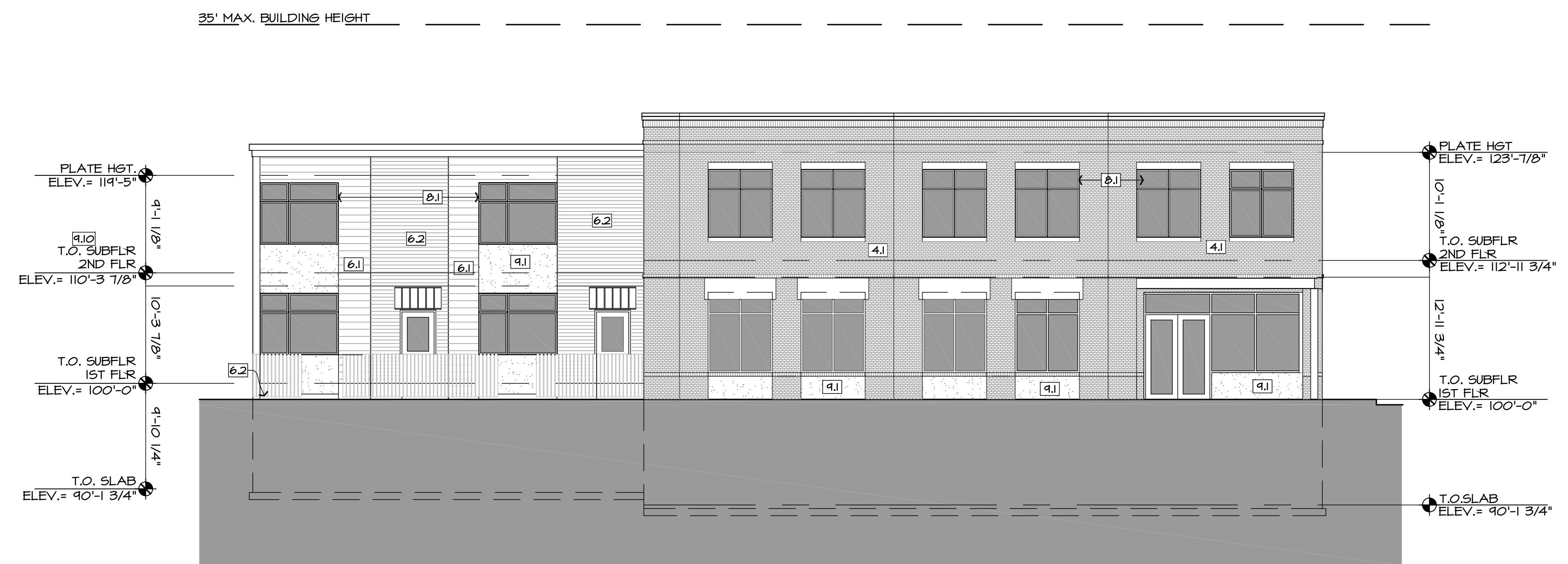
1 NORTH ELEVATION @ BUILDING A A2 SCALE: 1/8" = 1'-0"
